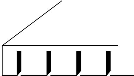
**Figure 3: Grid-Scored, Wide Cut (GSW) core material**
