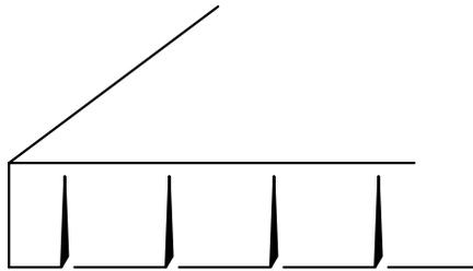
**Figure 4: Grid-Scored, Narrow Cut (GSN) core material**
