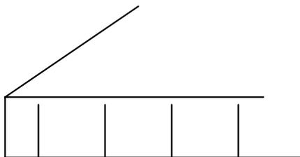
**Figure 5: Grid-Scored, Narrow Narrow Cut (GSNN) core material**
